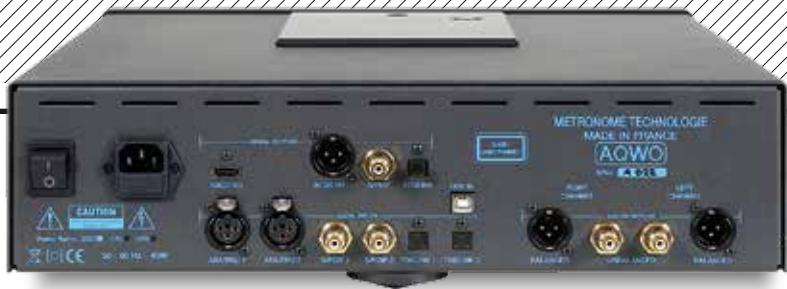
ABOVE: Two Toslink optical, two AES/EBU and two coaxial digital inputs are joined by an asynchronous USB-Type B. Outputs include single-ended on RCAs and balanced via XLRs, plus digital on Toslink, coaxial, AES/EBU and DSD as I 2 S on an HDMI socket
